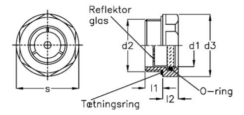
$\begin{array}{lll} d1 & = 32 \\ d2 & = G1 \ 1/4 \\ d3 & = 50 \\ I1 & = 12.0 \\ I2 & = 9.0 \\ Max \ pressure = 6 \ Bar \\ s & = 46 \end{array}$
